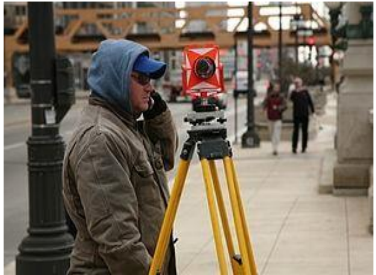
Fig. 7. A surveyor at work with an infrared reflector used for distance measurement
