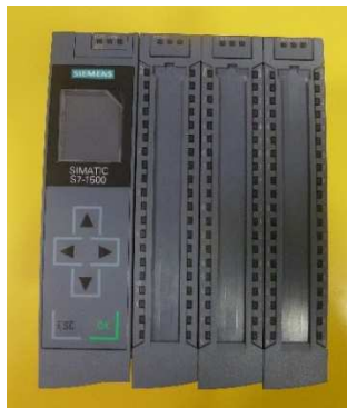
Fig. 12. PLC SIEMENS Simatic S7-1500 CPU 1512C-1PN
