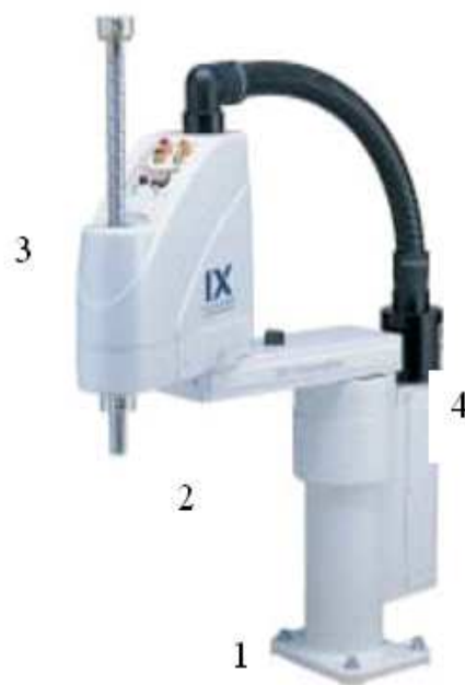
Fig. 5. Main parts of robot Scara
