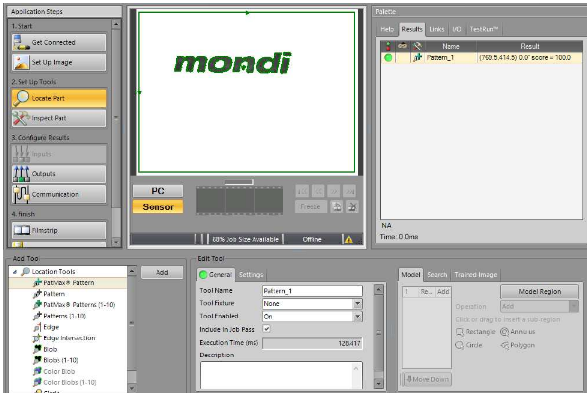
Fig. 6. Edge detection using PatMax
