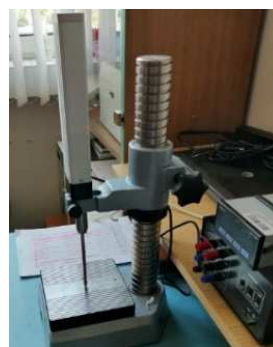
Fig. 2. Displacement sensor in comparator stand with digital counter
