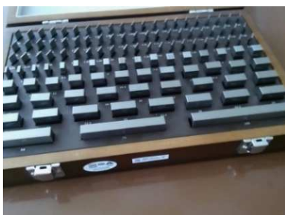
Fig. 3. Set of length gauge blocks (grade 0)
