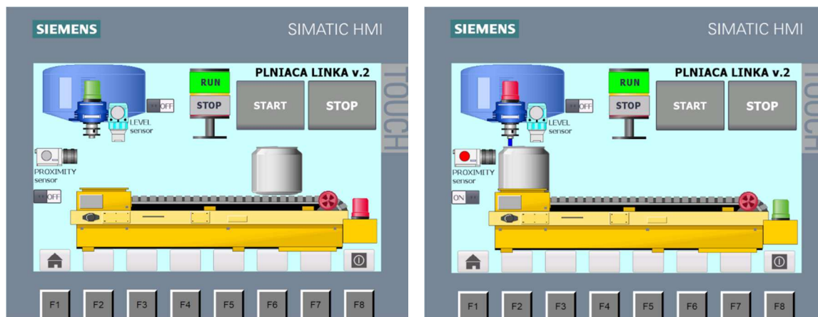
Fig. 13. Human machine interface for solved example of conveyor with tank and feed system
