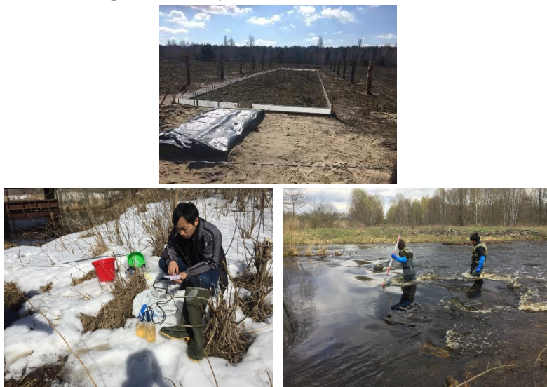
Fig. 3. One of the constructed experimental plots with the automatic gage system to measure soil erosion and radionuclide wash out from the watersheds; field measurements of the snowmelting runoff and collection of river flow data
