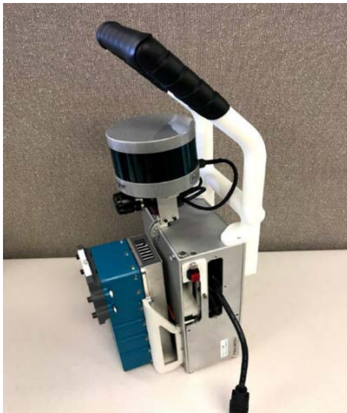
Figure 1: [Left] The Polaris-LAMP platform with LIDAR system (top), camera, coded aperture mask (grey) and detector module (blue).
