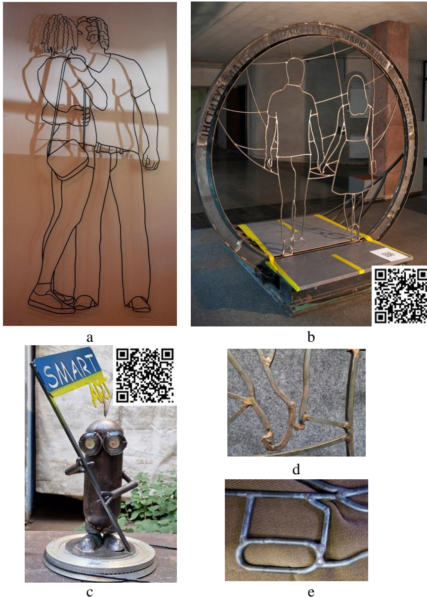
Fig. 1 – Sculptures with TIG braze welded joints produced in the workshop Smart Art (department of Welding Production of E.O. Paton Institute of Materials’ Science and Welding): a) “Macho”; b) “Into the Future!”; c) “Minion”; d) joints of wires 3, 4 and 5 mm dia e) joints of solid elements 10x10 mm
