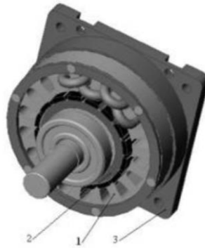
Fig. 1.1. Synchronous motor with permanent magnets
